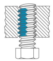
Tuflok® patches are well known for their cost benefits. They allow the same screw to be reused a number of times. As a result, maintenance and disassembly operations are simplified and cheaper.
