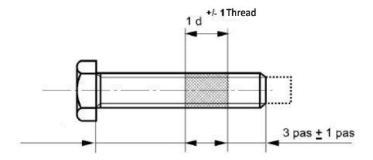
Note: When the thread is less than 1.25 in length and the diameter less than 8mm, the pre-coating length may be 0.6 to 0.8 times the diameter.
